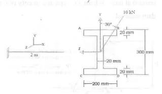
(c) Find torsion reactions at supports A & B for the given loading condition. Assume shear rigidity and uniform cross section.
