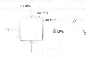
(c) A circle of 100 mm diameter is inscribed on a steel plate before it is stressed and then the plate is loaded as shown in figure. Then the circle is deformed into an ellipse. Determine the major and minor axes of the ellipse and their directions. Take  $E = 2.1 \times 10^6$
